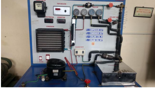
Fig.1 Photographic view of the experimental setup using R134a
